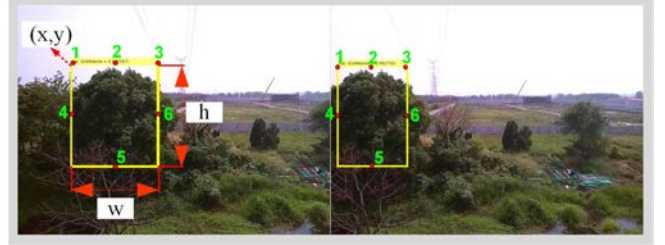
Fig. 8. Region detection of vegetation using Faster RCNN
