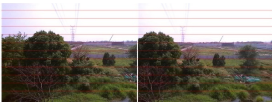
Fig. 7. Rectification of images with epipolar lines
